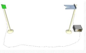
Next, rotate your test antenna to horizontal (while keeping the test distance constant) to measure the horizontal component of its gain. The two gains can be "power sum added" to come up with the AUT's total gain in the current test direction. Use the following formula:
