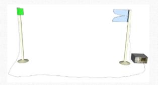
Now substitute your antenna under test (AUT) for one of your reference antennas. If the total patl loss increases by 2.5 dB, then your AUT has 2.5 dB less gain than your reference antenna. In this example, the AUT has an absolute gain of +3.7 dBi (at one frequency and in the tested direction). This is the vertical component of the AUT's gain.
